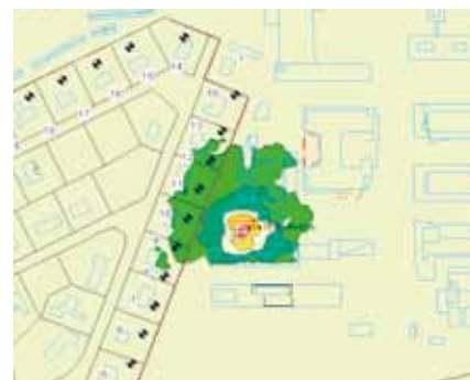
One of the messages from the local residents in Vosselaar resulted in the immediate noise remediation of the ventilators in Building 014 by the Engineering Department. A small adjustment to the ventilation settings had caused an unexpectedly large increase in the noise level. The sound cards provide a picture of the specific sounds of the building’s noise sources before (on the left) and after (on the right) the remediation was carried out.
