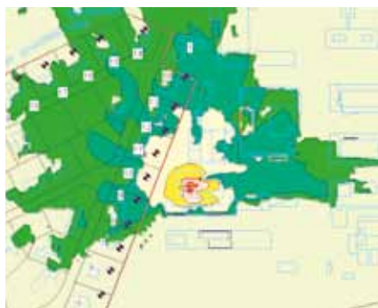
One of the messages from the local residents in Vosselaar resulted in the immediate noise remediation of the ventilators in Building 014 by the Engineering Department. A small adjustment to the ventilation settings had caused an unexpectedly large increase in the noise level. The sound cards provide a picture of the specific sounds of the building’s noise sources before (on the left) and after (on the right) the remediation was carried out.
