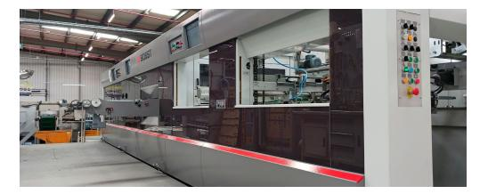
We replaced the two old machines with one flatbed die-cutter. Not just any one, but really the Rolls Royce among die-cutters. The machine can output as many as 7.500 sheets per hour. Moreover, it can process sheets with a maximum size of 1450 x 1050 mm.
